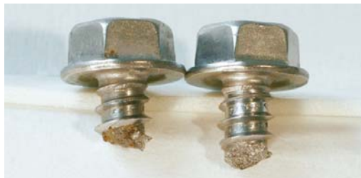
Example of how fasteners can fail due to hydrogen-assisted cracking (HAASCC). These 410 SS super passivated fasteners with plain finish (above) and 410 fasteners with aluminum-filled topcoat (below) failed at the interface of the aluminum and steel sheets during salt spray tests.
