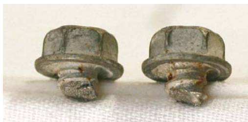
Example of how fasteners can fail due to hydrogen-assisted cracking (HAASCC). These 410 SS super passivated fasteners with plain finish (above) and 410 fasteners with aluminum-filled topcoat (below) failed at the interface of the aluminum and steel sheets during salt spray tests.
