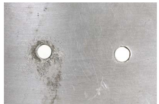
Unplated 300 series stainless screws vs. fasteners with Stalgard GB were installed side-by-side in aluminum plate and put into salt spray testing for 1000 hours per ASTM B117.
