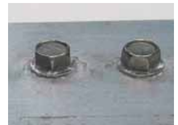
The Bi-Flex fasteners did not fail and did not lose preload.
