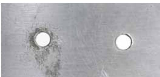
The modified 400 SS fasteners, 410 SS super passivated fasteners with plain finish, and 410 fasteners with aluminum-filled topcoat failed at the interface of the aluminum and steel or directly under the fastener head.
